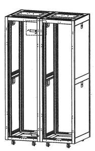
Fix the bracket to the top and bottom of the front and rear rack frame posts.
